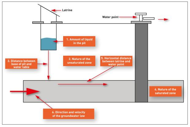
Figure 1. Six different factors which can effect pathogen transmission from a latrine to a nearby water point
