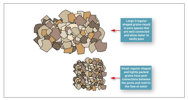
Figure 2. Volume of the spaces (or pores) between the grains
